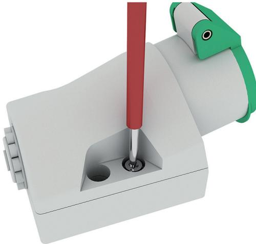
3. Loosen the screws of the terminals with a screwdriver and pull out the individual conductors from the terminals.
